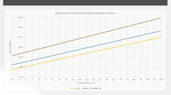
When the amount of air molecules doesn't change in a tyre, then the pressure is proportional to the temperature, as the volume stays constant. An important remark is that temperature has to be measured in degrees Kelvin and not in degrees Celsius or Fahrenheit. The unit for the pressure does not matter.
